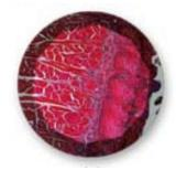
5. "The field diaphragm is now opened until about three-quarters of the viewfield is visible and the condenser is then refocused. Check alignment of the condenser and re-adjust if necessary."
